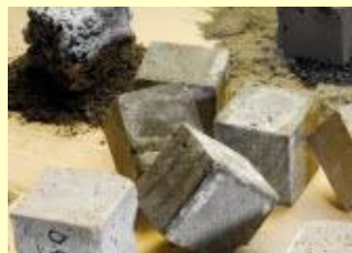
Pieces of Wallboard made from coal ash
